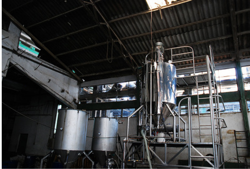
Photo 2: The technology to separate the fish gut from water and adding methanol to produce the bio-diesel (Aquafinca, Honduras)
